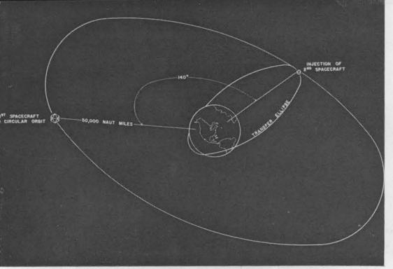
DETECTION SATELLITES' orbits are shown in this drawing. From the transfer ellipse, both satellites were accelerated into the circular orbit, but the second followed the first after traveling the transfer ellipse twice, some 40 hours later.
